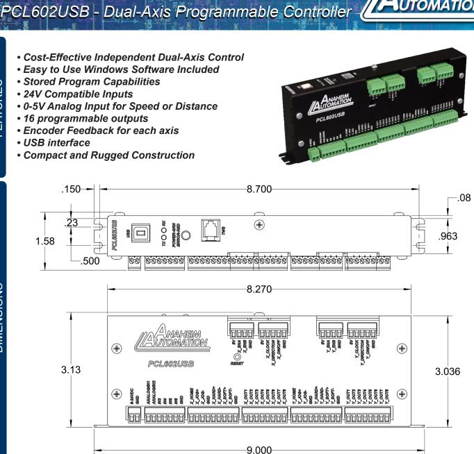
The PCL602USB is a dual-axis step motor controller containing 2 Kbytes of nonvolatile stored programming space and quadrature encoder feedback. This device provides flexible and independent control of two stepper motors from computers or any machine controller with a USB port. More specifically, the PCL602USB presents an easy way to implement motion systems requiring two axes and the precision that can be achieved on each axis through the use of encoder feedback.
